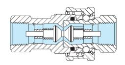
HK Couplings are so designed that, when the coupling is being connected, the seal is made before the valves open to allow fluid to flow. On disconnection the valves close to seal off both ends of the line before the main coupling seal is broken.
