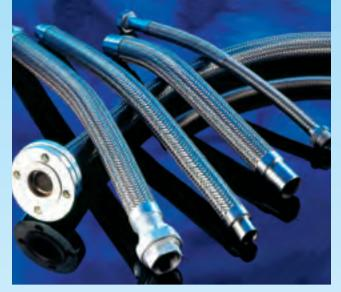
Design & Installation: Kaptech Stainless Steel flexibles should be configured and installed in such a way that the minimum bend radius is not exceeded, the hose is not stretched, compressed nor twisted, and the external braid is not subject to wear nor damage. The use of elbow ends can often help in achieving a
