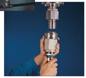
requirements. They can be used for connecting a flexible hose to a fixed pipe, vessel, cylinder, etc., connecting a hose between two fixed points, plugging-in an instrument (e.g. a pressure gauge) to test points, or connecting two hoses together. Where one hose may need to be connected to several outlets, or several hoses to one outlet, the hoses or outlets not in use remain automatically sealed.
