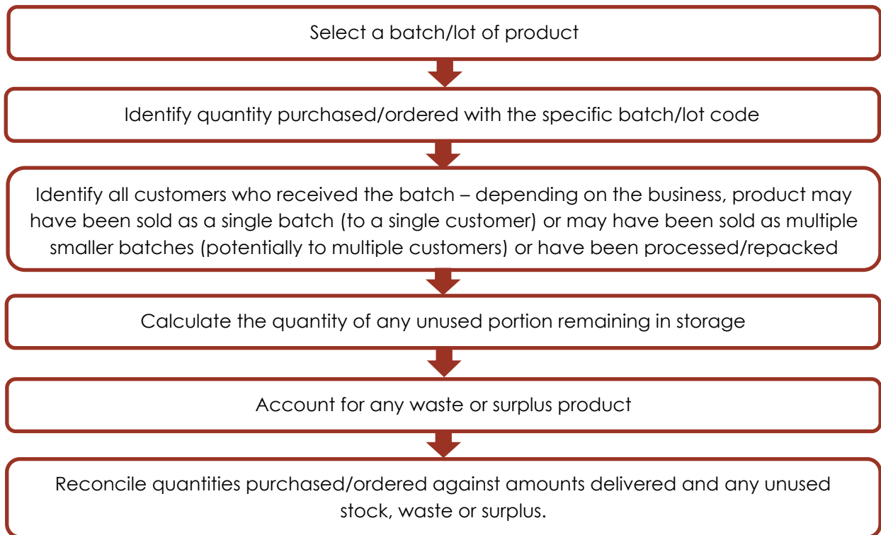
Figure 7: Mass balance calculation process
