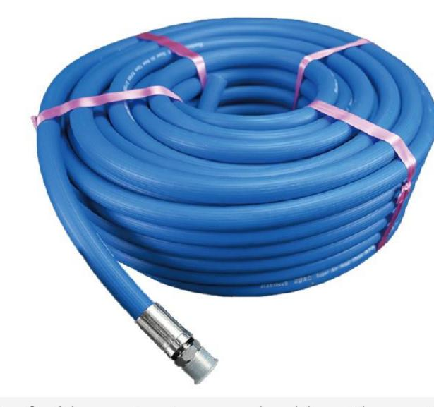
Two kinds of rubber water pipes are durable, with an outer diameter of 20mm and an inner diameter of 13mm. High pressure resistant, can be used with high-pressure water gun and water pipe rack.
