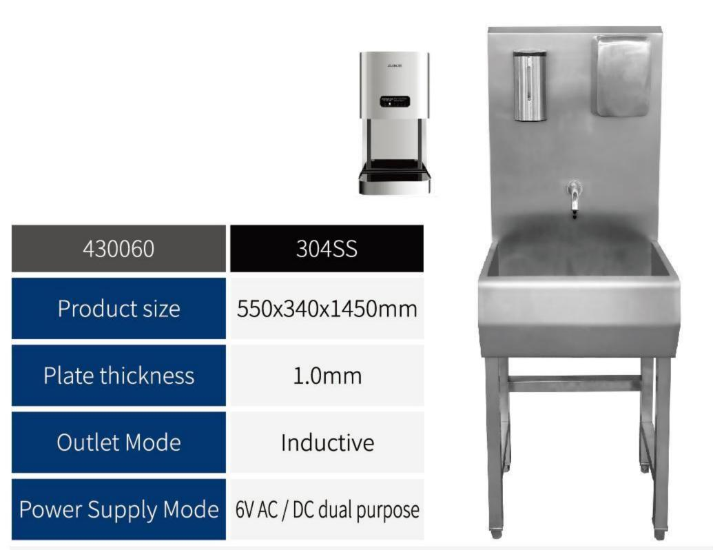
304 stainless steel hand washing and disinfection station, consisting of an induction water tank, soap dispenser, hand dryer, and alcohol sterilizer, integrates to complete the entire process of hand washing and disinfection.
